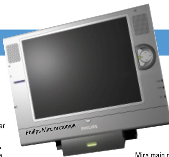
base and used anywhere in the house. When it's mobile, it communicates with the PC via WiFi (802.11b) wireless. Most of the
