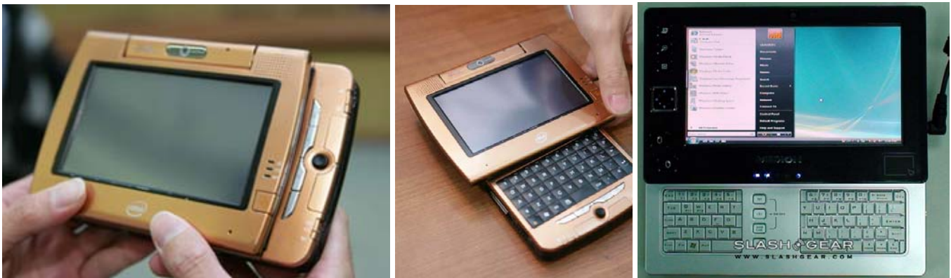
Left image: Quanta 's prototype UMPC based on Intel's reference design; center image: Quanta 's prototype with the keyboard rotated and opened; right image: The Medion MD RIM 1000, shown with the sliding keyboard extended
